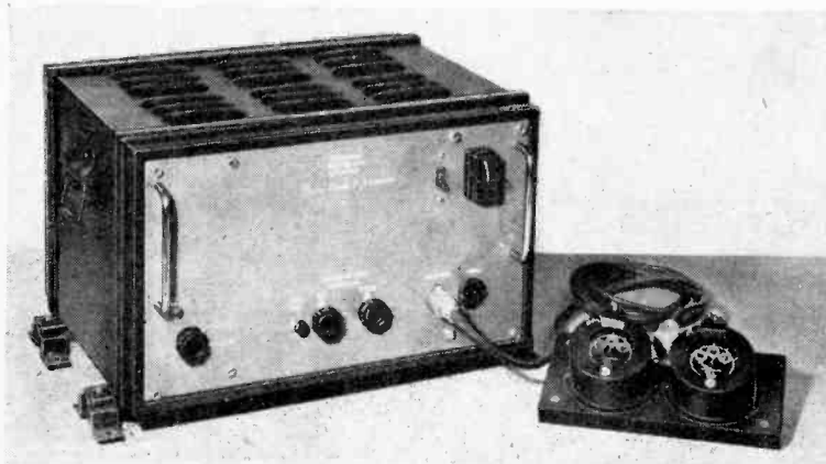
A marine model of the Decca Navigator.
